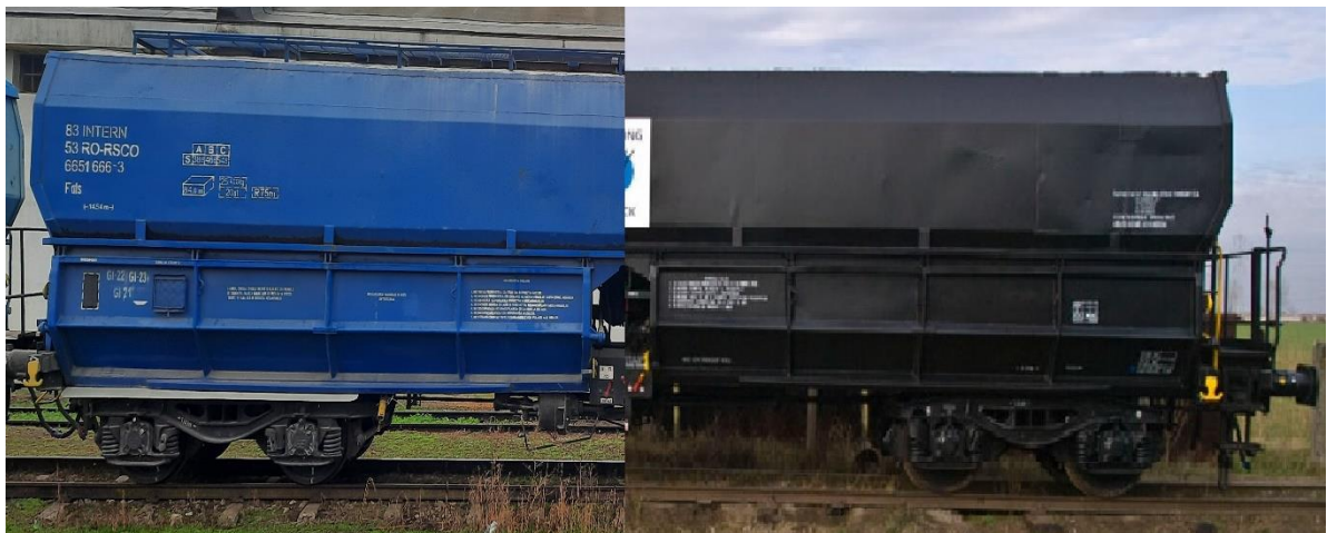
Photo no. 9 - Fals series wagon with fixed down-grade compared with Fals series wagon without this extension.
