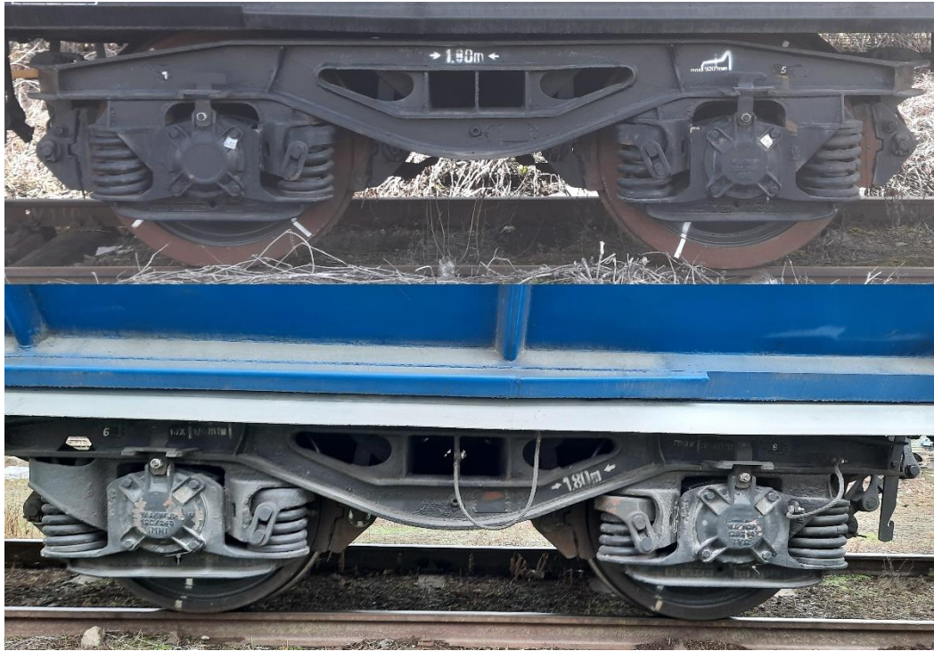
Photo nr.10 - Comparative photo of the access to the side bearers of the Fals series wagon (top) and the Fals series wagon with fixed down-grade (bottom)
